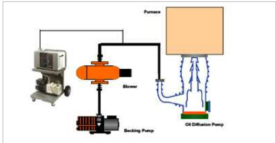
*Helium leak detection arrangement on a furnace*
