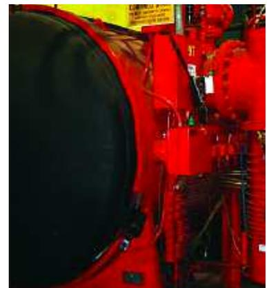
vacuum applications, a vacuum decay rate above 10 microns/hour in the heating chamber is unacceptable.
